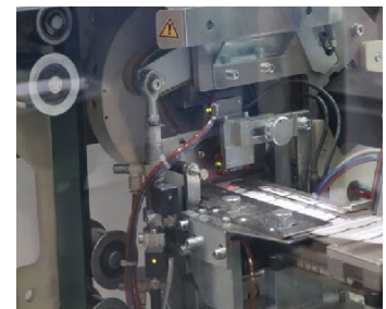
Fujitsu RFID tag on roll and being inserted into linen during Venus Group automation process
